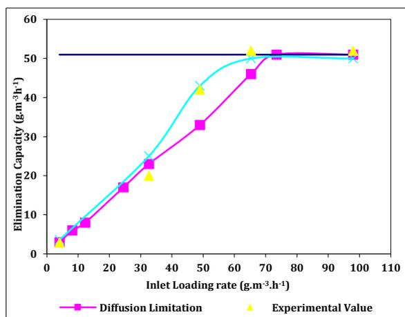
Fig. 8 Comparison of ottengraf model and modified ottengraf model with experimental values for MEK removal in a cornstack based biofilter.
