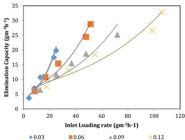
Fig. 6 Inlet Load Vs Elimination capacity for the removal of MEK using Press mud based biofilter
