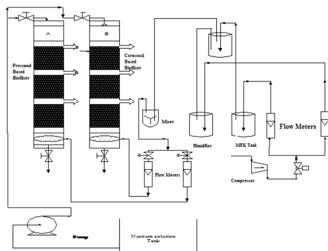
Fig. 1 Schematic diagram of biofilter
