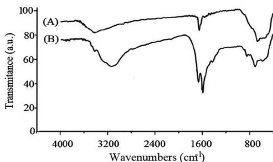
Fig. 4 FTIR image of (a) pure TiO<sub>2</sub> and (b) dyed TiO<sub>2</sub>
