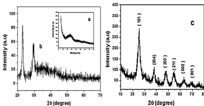
**Fig. 2** PXRD patterns of (a) pure TiO<sub>2</sub> (b) dyed TiO<sub>2</sub> (c) dyed TiO<sub>2</sub> after calcinations at 250 °C
