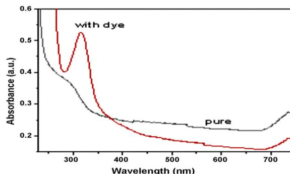
**Fig. 1** UV visible patterns of (a) pure TiO<sub>2</sub>, (b) dyed TiO<sub>2</sub>
