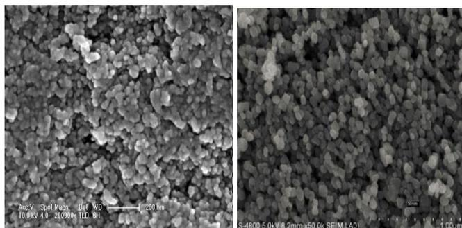
Fig. 3 SEM image of (a) pure TiO<sub>2</sub> and (b) dyed TiO<sub>2</sub>
