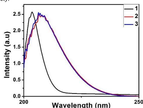
Fig. 1 Absorption spectrum of the ZnO 40 °C sol, 50 °C sol and 60 °C sol, respectively, are indicated by the graphs "1", "2" and "3".
