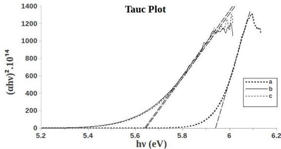
**Fig. 2** Tauc plot of the 40 °C sol, 50 °C sol and 60 °C sol, respectively, are indicated by the graphs "a", "b" and "c". The straight line in the plot are Tauc's extrapolation straight line.
