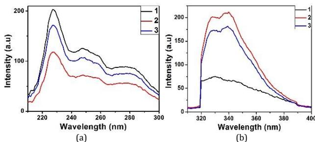
**Fig. 3** a) The graphs 1,2,3 are excitation spectrum of the ZnO 40 °C sol, 50 °C sol and 60 °C sol, respectively, obtained by monitoring emission at 330 nm. b) The graphs 1,2,3 are emission spectrum of the ZnO 40 °C sol, 50 °C sol and 60 °C sol, respectively, obtained while the sols were excited at 227 nm
