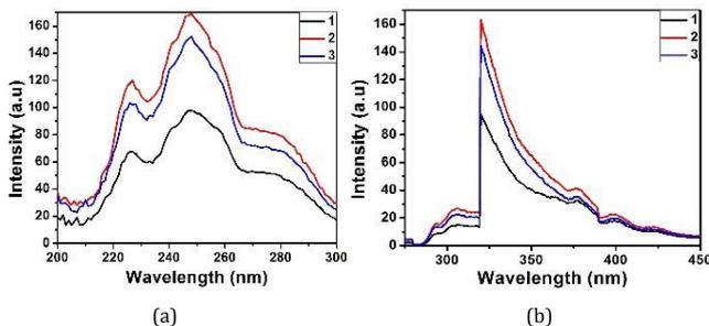
**Fig. 4** a) The graphs 1,2,3 are excitation spectrum of the ZnO 40 °C sol, 50 °C sol and 60 °C sol, respectively, obtained by monitoring emission at 320 nm. b) The graphs 1,2,3 are emission spectrum of the ZnO 40 °C sol, 50 °C sol and 60 °C sol, respectively, obtained while the sols were excited at 250 nm
