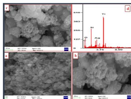
Fig. 1 SEM image for TiO<sub>2</sub> (a) TiO<sub>2</sub>@SiO<sub>2</sub>-Ag (b, c) and (d) EDX- Spectrum of elemental analysis
