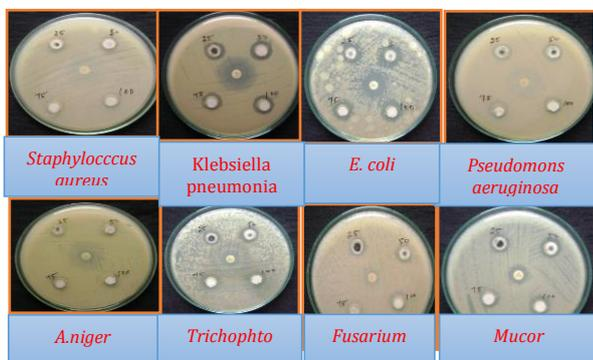
Fig. 2 Bactericidal and fungal activity assay by  $\text{TiO}_2@SiO_2\text{-Ag}$  nanocomposite
