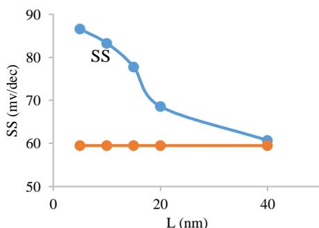
**Fig. 4** SS with channel length of Si-FinFET
