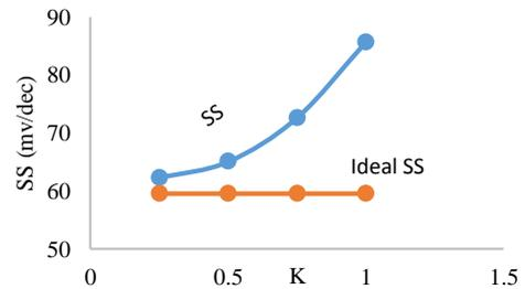
Fig. 13 SS with scaling factor (K) of Si-FinFET
