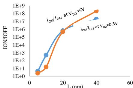
**Fig. 3**  $I_{ON}/I_{OFF}$  ratio with channel length of Si-FinFET
