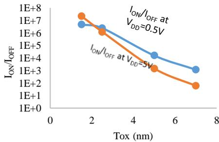
Fig. 9  $I_{ON}/I_{OFF}$  with oxide thickness of Si-FinFET
