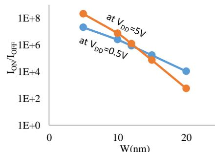
**Fig. 6**  $I_{ON}/I_{OFF}$  with channel width of Si-FinFET
