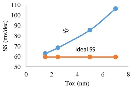
Fig. 10 SS with oxide thickness of Si-FinFET
