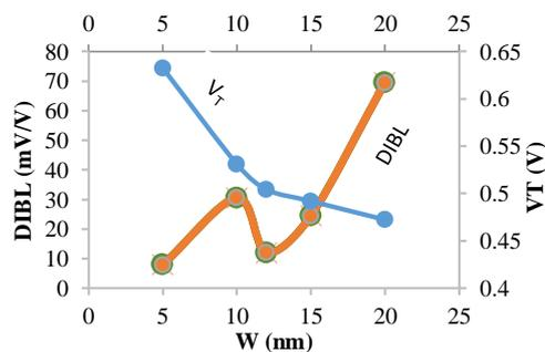
**Fig. 8**  $V_T$ , DIBL with channel width of Si-FinFET
