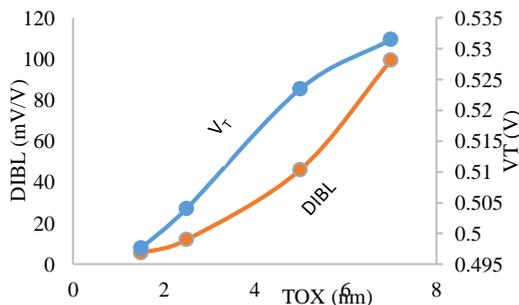
Fig. 11  $V_T$ , DIBL with channel oxide thickness of Si-FinFET
