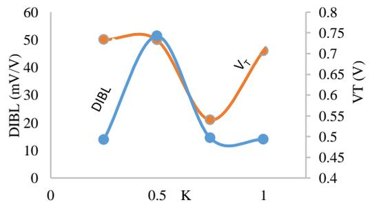
Fig. 14  $V_T$  and DIBL with scaling factor (K) of Si-FinFET
