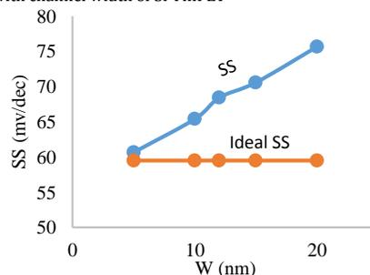
**Fig. 7** SS with channel width of Si-FinFET
