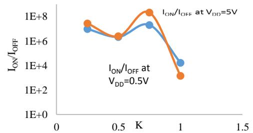
Fig. 12  $I_{ON}/I_{OFF}$  with scaling factor (K) of Si-FinFET
