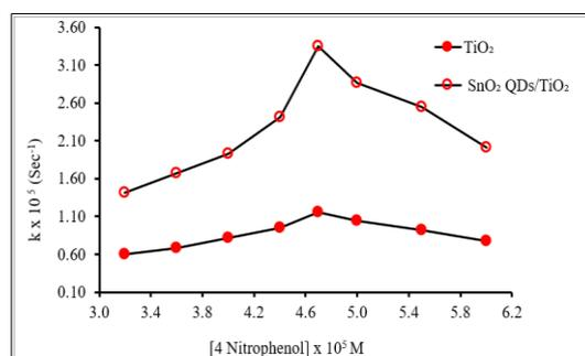
Fig. 5 Variation of rate constant with concentration of 4-nitrophenol (pH = 8.0, Semiconductor = 0.10 g, Light intensity =  $50.0 \text{ mWcm}^{-2}$ )
