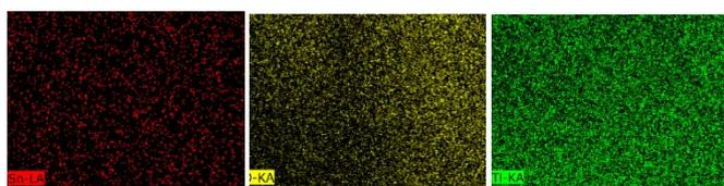
Fig. 2 EDX mapping image of  $\text{TiO}_2/\text{SnO}_2$  QDs composite
