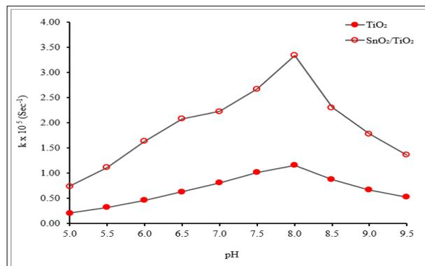
Fig. 4 Variation of rate constant with pH ([4-NP] =  $4.7 \times 10^{-5}$  M, Semiconductor = 0.10 g, Light intensity =  $50.0 \text{ mWcm}^{-2}$ )
