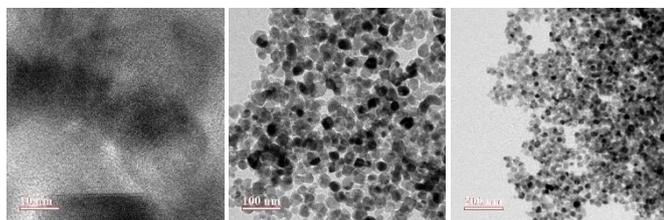
Fig. 1 HRTEM images of  $\text{TiO}_2/\text{SnO}_2$  QDs Composite
