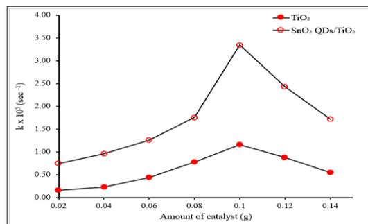
Fig. 6 Variation of rate constant with amount on photocatalyst (pH = 8.0, [4-NP] =  $4.70 \times 10^{-5}$  M, Light intensity =  $50.0 \text{ mWcm}^{-2}$ )
