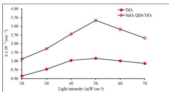
Fig. 7 Variation of rate constant with light intensity (pH = 8.0, [4-NP] = 4.70 × 10<sup>-5</sup> M, Semiconductor = 0.10 g)
