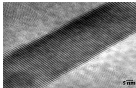
Fig. 3 The HRTEM image of Fe-TiO<sub>2</sub> nanoparticles
