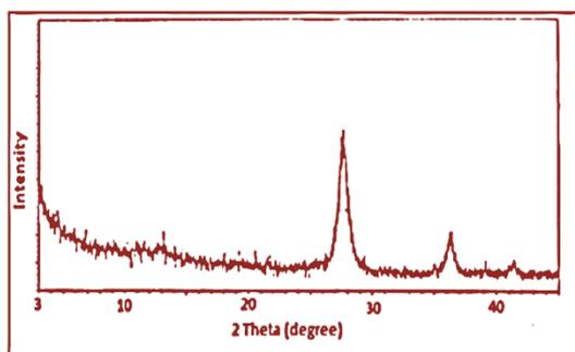
Fig. 1 XRD pattern of Fe-TiO<sub>2</sub> nanoparticles
