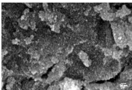
Fig. 8 The HRTEM image of NiFe<sub>2</sub>O<sub>4</sub> NPs
