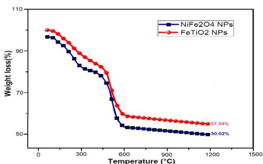
Fig. 9 TGA curve of NPs
