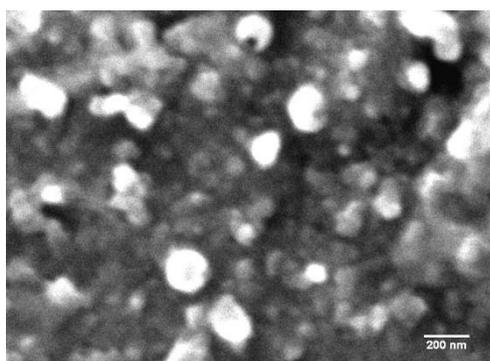
Fig. 2 FESEM Image of Fe-TiO<sub>2</sub> nanoparticles
