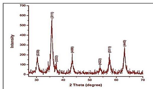
Fig. 5 XRD pattern of NiFe<sub>2</sub>O<sub>4</sub> nanoparticles
