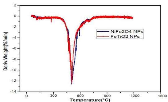
Fig. 10 DTG curve of NPs
