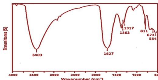
Fig. 6 FTIR spectra of NiFe<sub>2</sub>O<sub>4</sub> NPs
