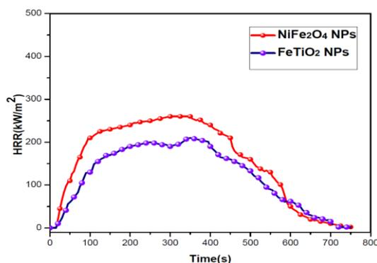
Fig. 11 PHRR curves of NPs
