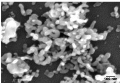
Fig. 7 FESEM image of NiFe<sub>2</sub>O<sub>4</sub> NPs
