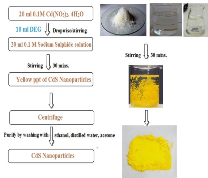
Fig. 1 Schematic illustration of the aqueous precipitation synthesis of CdS nanoparticles
