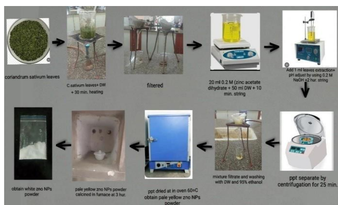
Fig. 1 The schematic way of synthesis of zinc oxide nanoparticles (ZnONPs)
