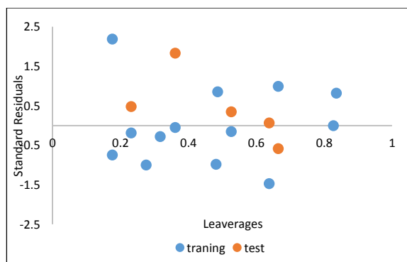
Fig. 5 The Williams plot, the plot of the standardized residuals versus the leverage value for training and test set
