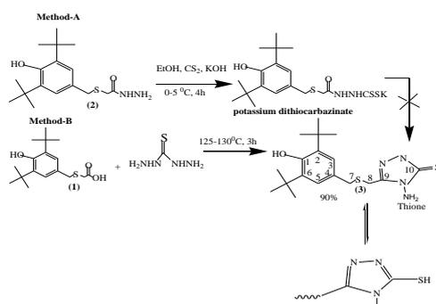
**Fig. 4** Synthetic scheme for the formation of 4-amino-3-((3,5-di-tert-butyl-4-hydroxybenzylthio) methyl)-1H-1,2,4-triazole-5(4H)-thione(1) [35]
