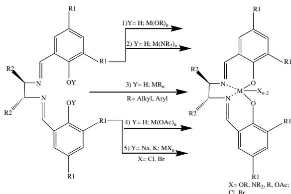
**Fig. 2** Preparation of metal complexes of Schiff bases [33]
