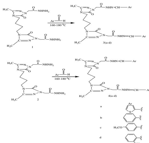
**Fig. 5** Synthetic pathway for the preparation of compounds 3-4(a-d) [42]
